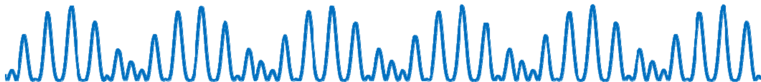
Typical detector signal containing 4, 40, and 44 MHz contributions
